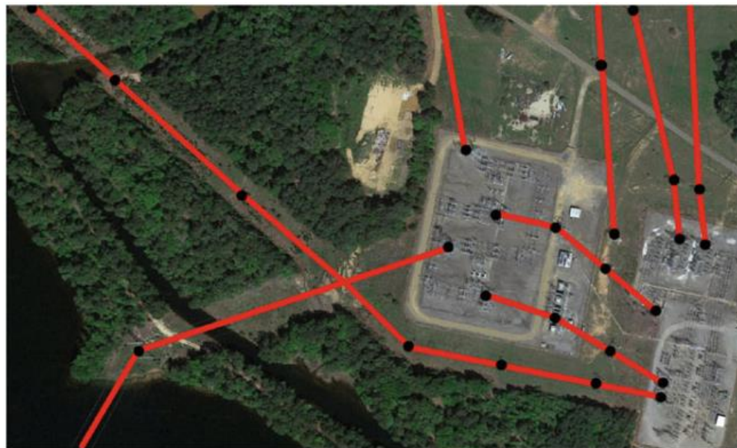
Fig. 2 Tracing transmission lines on GIS services
