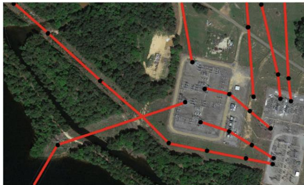
Fig. 2 Tracing transmission lines on GIS services
